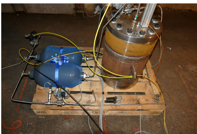
Fig. 1. View and scheme of the experimental setup of the explosion vessel
