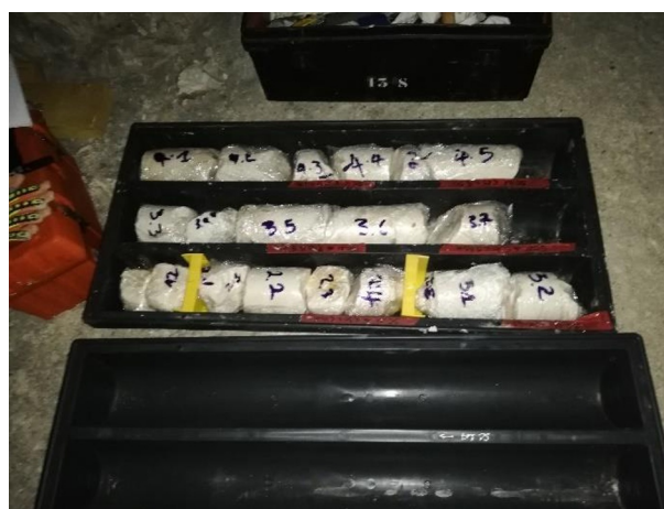
Figure 2. Chalk cores drilled from the Royer mine
