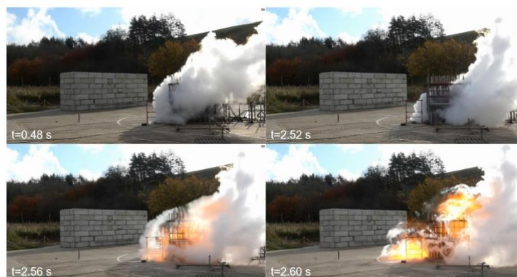
Figure 5. Stills images showing sudden gust immediately prior to ignition in Trial 23 [34].
