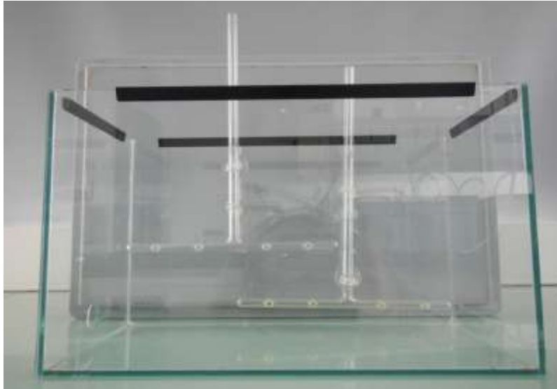
Figure S2 Two diffusion ramps and an aquarium used in the experiments (20*40*25 (w*L*h) cm, 20 L)
