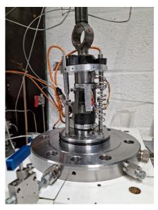
Figure 2. Local deformation measurement system.
