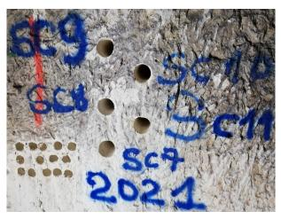
Figure 1. Plugs cored from pillars in the Royer mine.
