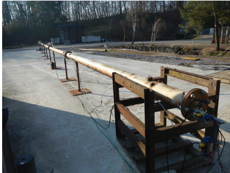
Fig. 1. View of the experimental set-up. Steel pipe, with a 150-mm inner diameter.
