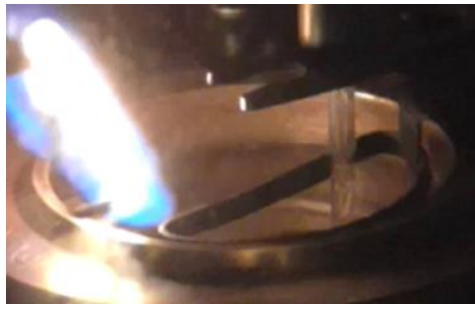
Fig 6.: Pilot flame above the liquid ethoxy-nonafluorobutane at a temperature of 32°C
