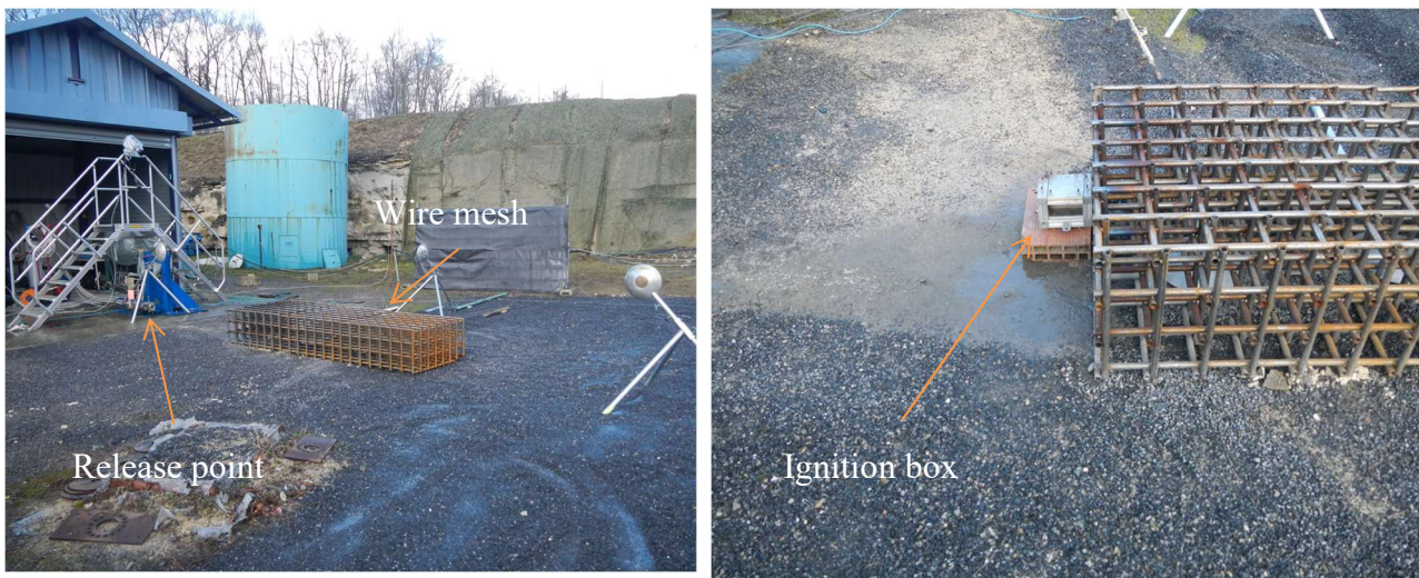
Fig. 7. Experimental configuration and ignition box
