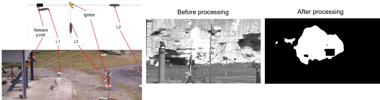
Fig. 3. Overall repartition of pressure gauges and flame image processing
