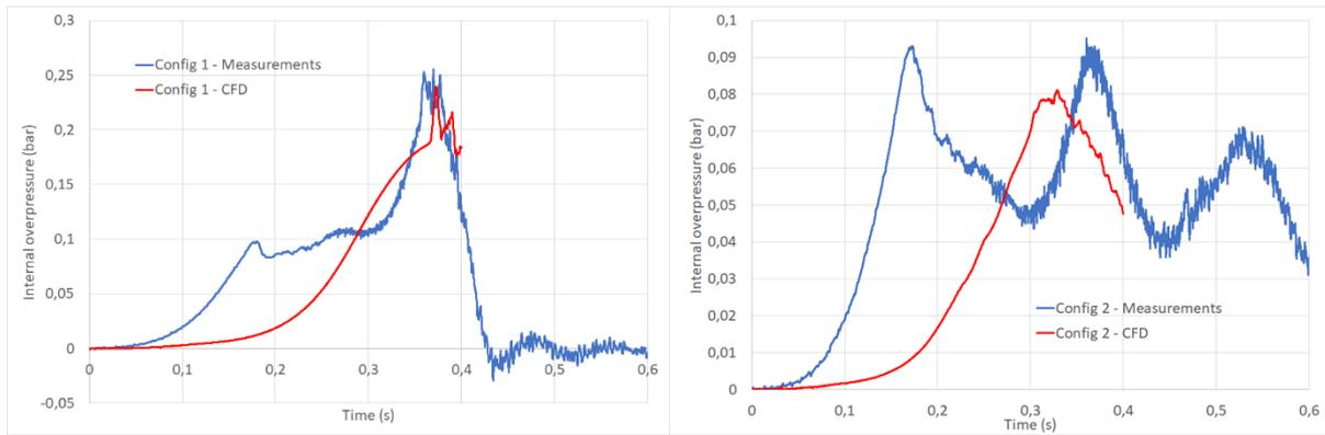
**Fig. 7.** Comparison of the measured and computed pressure signals inside the 37 m<sup>3</sup> enclosure for the two configurations.
