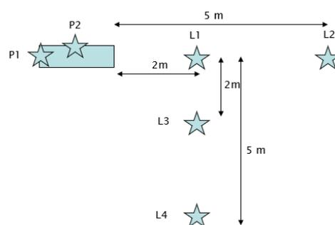
**Fig. 1.** Locations of the pressure sensors for the 4 m<sup>3</sup> enclosure. View from the top.
