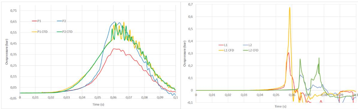
**Fig. 4.** Case of the initially quiescent mixture with a hydrogen volume fraction of 21 %. Comparison of the computed and measured pressure signals inside ou outside the 4 m<sup>3</sup> enclosure.
