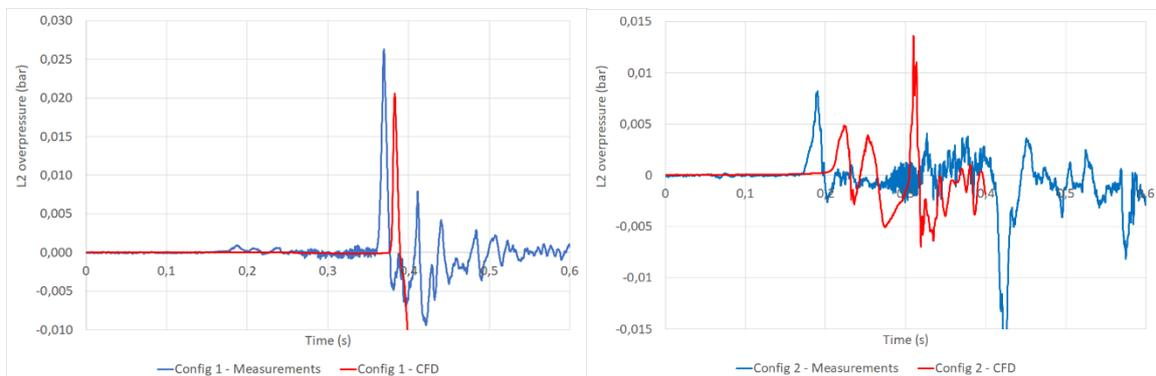
**Fig. 9.** Comparison of the measured (left) and computed (right) pressure signals at the pressure probe L2 outside the 37 m<sup>3</sup> enclosure for the two configurations.
