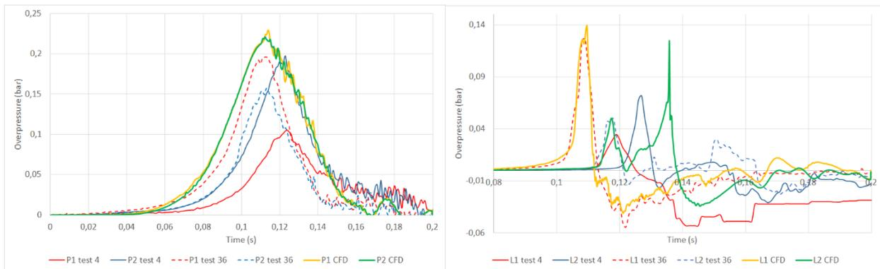
**Fig. 3.** Case of the initially quiescent mixture with a hydrogen volume fraction of 16 %. Comparison of the computed and measured pressure signals inside (left) ou outside (right) the 4 m<sup>3</sup> enclosure.
