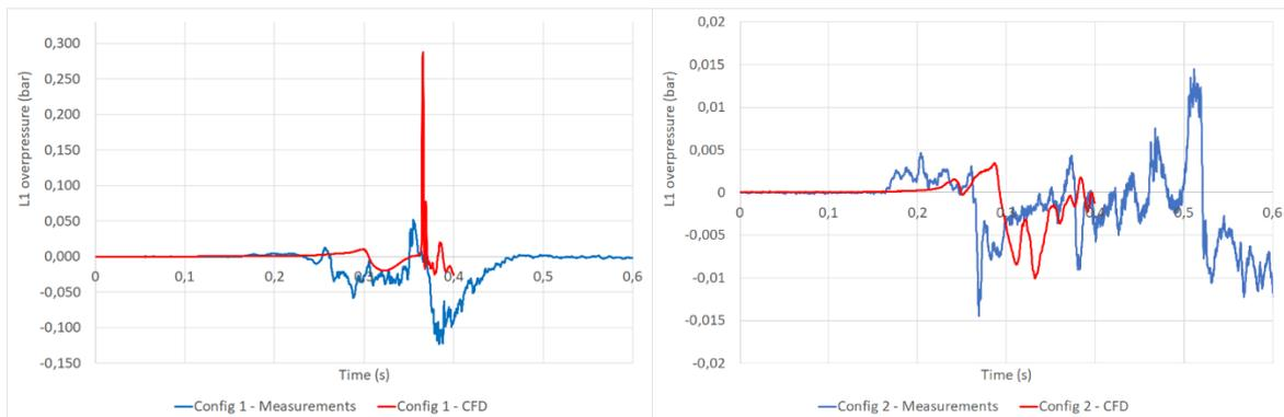
**Fig. 8.** Comparison of the measured and computed pressure signals at the pressure probe L1 outside the 37 m<sup>3</sup> enclosure for the two configurations.
