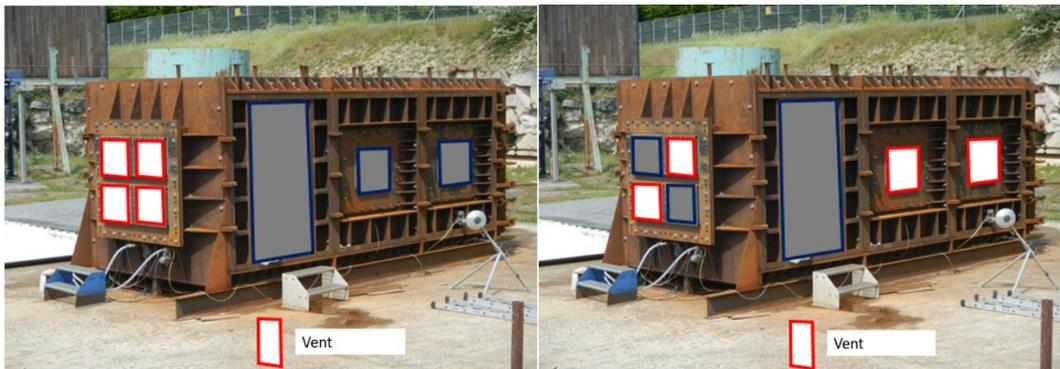
**Fig. 2.** View of the 37 m<sup>3</sup> enclosure and of the possible locations of the vents (in red). Left: configuration 1, right: configuration 2. Panels in blue are safety vents which should not open during the explosion.
