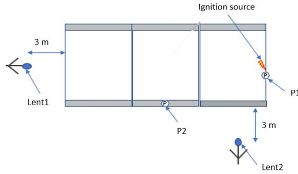
**Fig. 3.** Location of the ignition source and pressure sensors for the 37 m<sup>3</sup> confined explosions (P1, P2: inside pressure – Lent1, Lent2: outside pressure)
