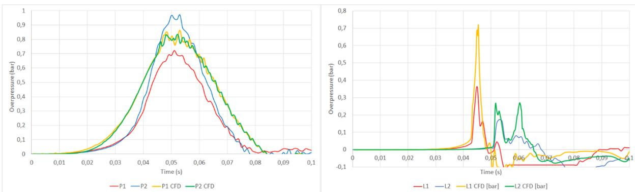
**Fig. 5.** Case of the initially quiescent mixture with a hydrogen volume fraction of 25 %. Comparison of the computed and measured pressure signals inside ou outside the 4 m<sup>3</sup> enclosure.
