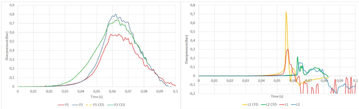
**Fig. 6.** Case of the initially turbulent mixture with a hydrogen volume fraction of 21 %. Comparison of the computed and measured pressure signals inside (left) and outside (right) the 4 m<sup>3</sup> enclosure.
