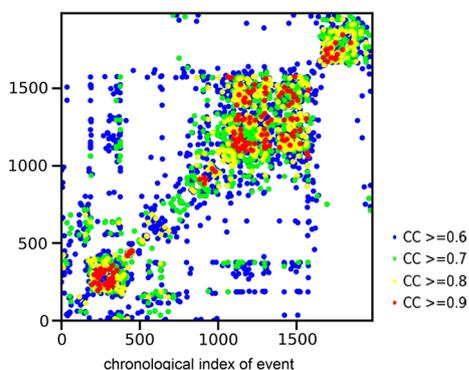
**Fig. 4** Crosscorrelation matrix showing cross-correlation values, for all event pairs calculated as a mean value across all 3 components. Only event pairs with crosscorrelation values of 0.6 and higher are shown (adapted from Namjesnik 2021)
