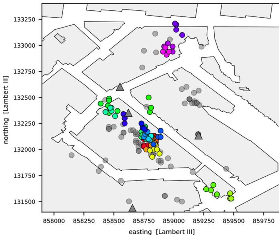
**Fig. 6** Location of events of main multiplet families with more than 3 events. Grey circles indicate higher magnitude events ( $M_w > 1$ ) that are not part of multiplet families (adapted from Namjesnik 2021)
