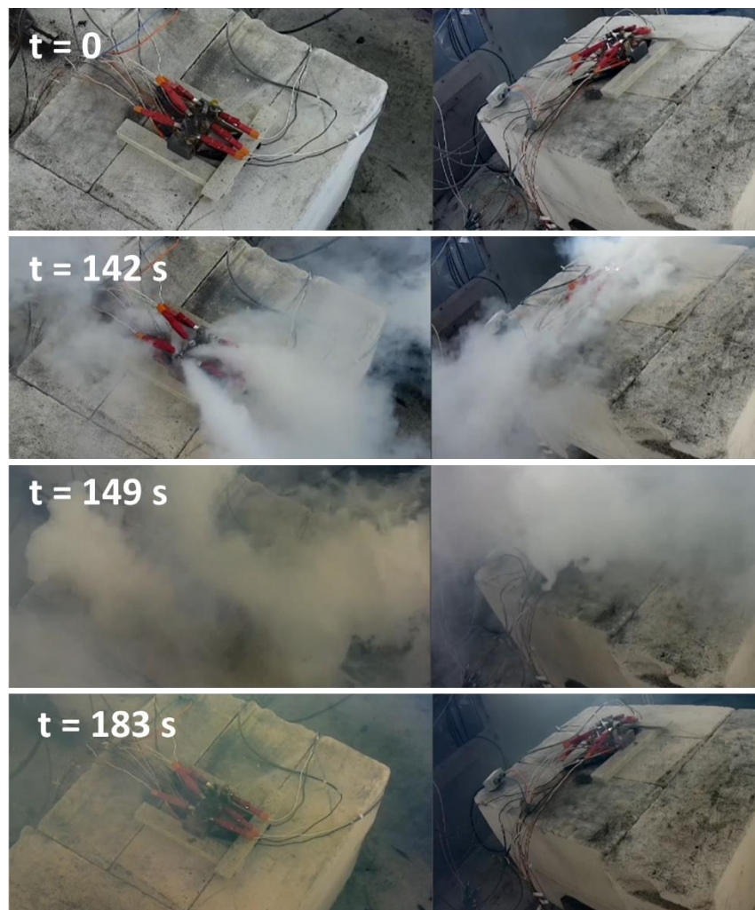
Figure 3: Extract from the video of the test before, during and after thermal runaway
