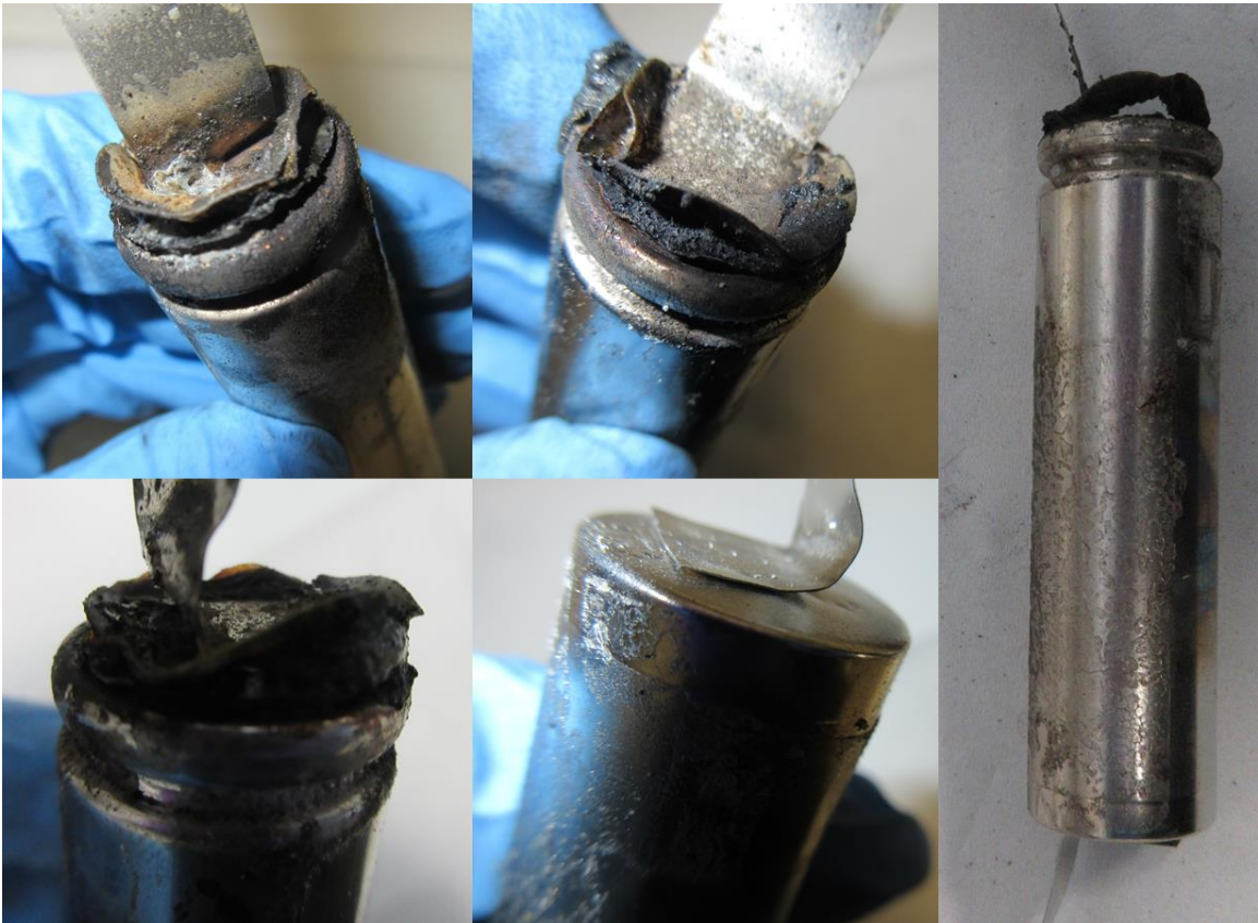
S4 : Visual observation of thermal runaway induced degradation in four of the six tested cells.
