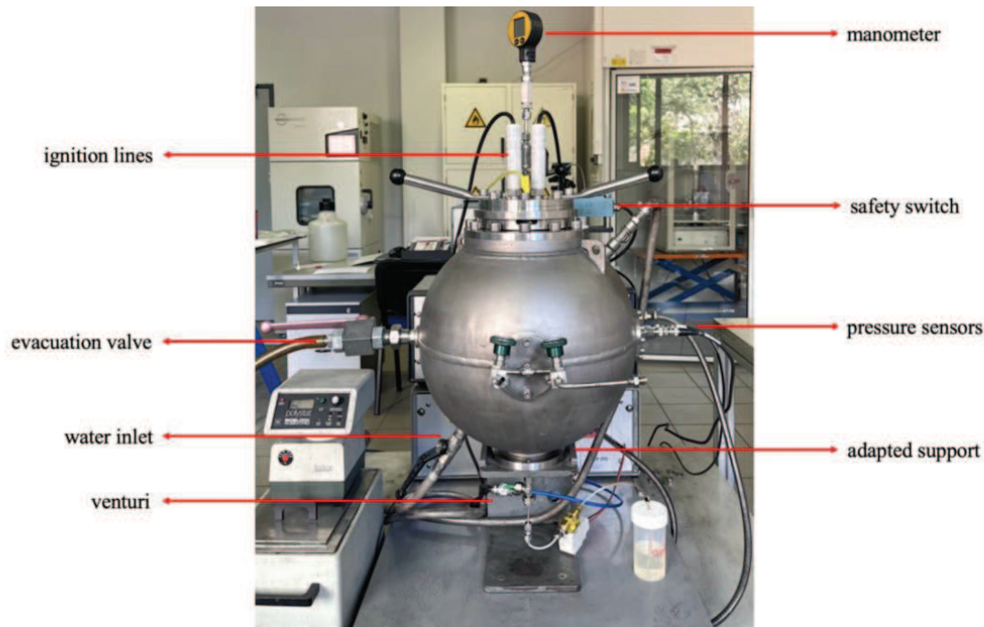
Figure 3: The Modified 20 L Ignition and explosion Severity Test device
