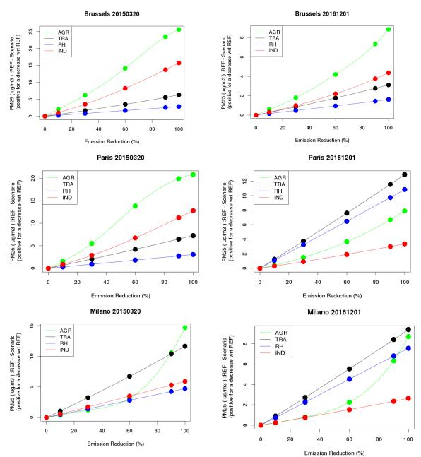
Figure S1 : Modelled PM<sub>2.5</sub> reduction (y-axis : positive for a decrease with respect to the reference,  $\mu g/m^3$ ) for a given reduction in Agriculture (green), Industrial (red), Residential Heating (blue), and Traffic (black) emissions (x-axis: in %) in Brussels, Paris and Milano (top to bottom) and for 20150320 (left) and 20161201 (right).
