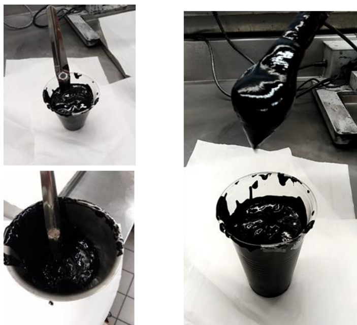
Figure 31: Lab scale preparation of electrode ink.
