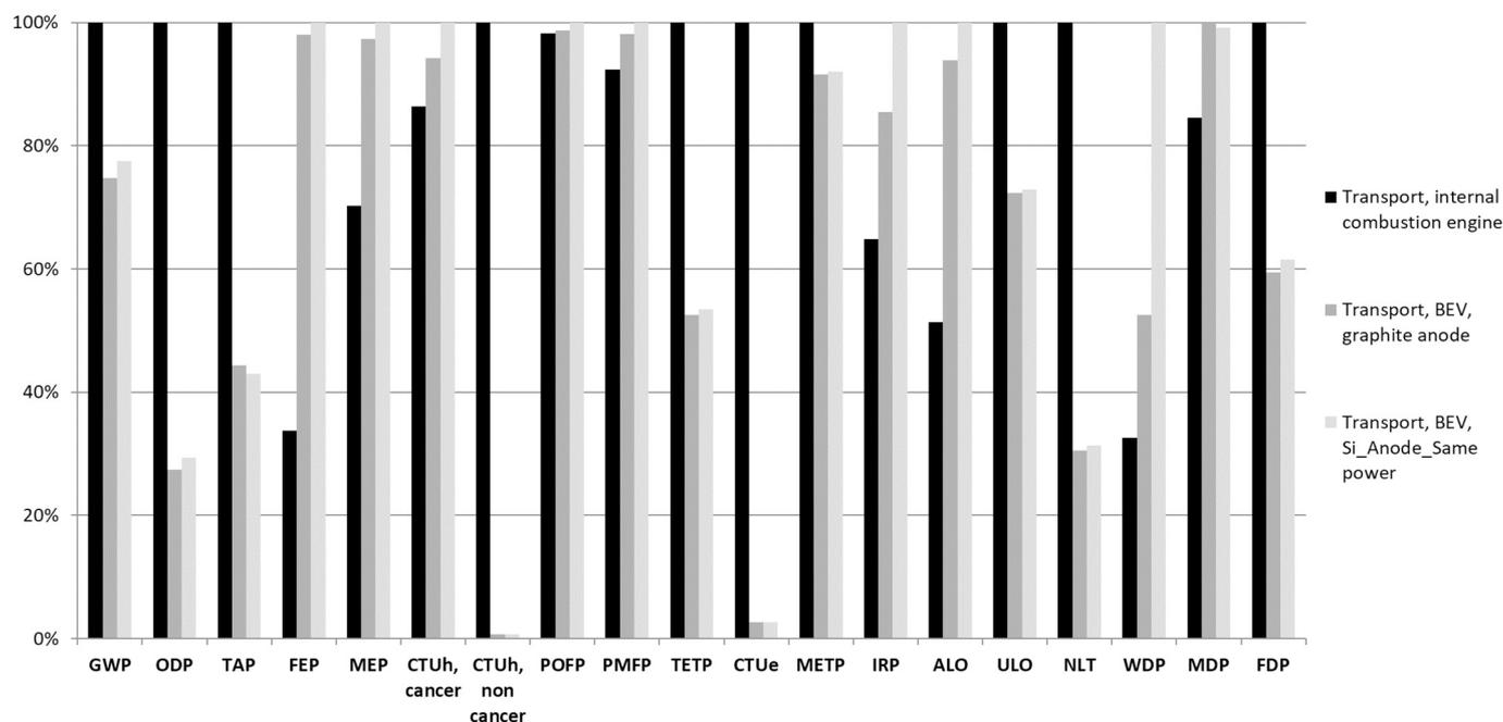
**Fig. 4.** Environmental impacts of driving 1 km with a passenger car with an internal combustion engine, with a BEV using a Li-ion battery containing Si 40 nanoparticles in the anode and with a BEV using a Li-ion battery with a graphite based anode. The highest value is each time set as 100%. Shown are the same midpoint indicators as in Fig. 2.
