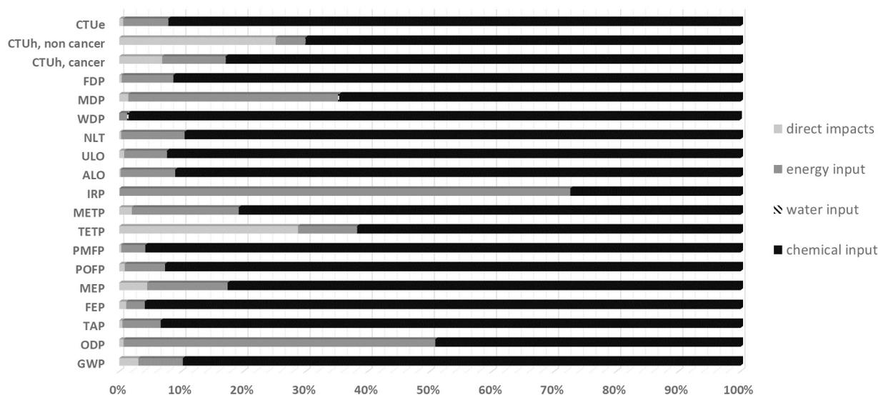
**Fig. 2.** Environmental impacts of the production of 1 kg of Si 40 nm. Reported are the relative contributions of the various inputs and of direct emissions (including the production of waste treated in the waste treatment activities). These results are shown using various ReCiPe midpoint indicators, except for the toxic impact categories, where the USEtox midpoint indicators are applied.
