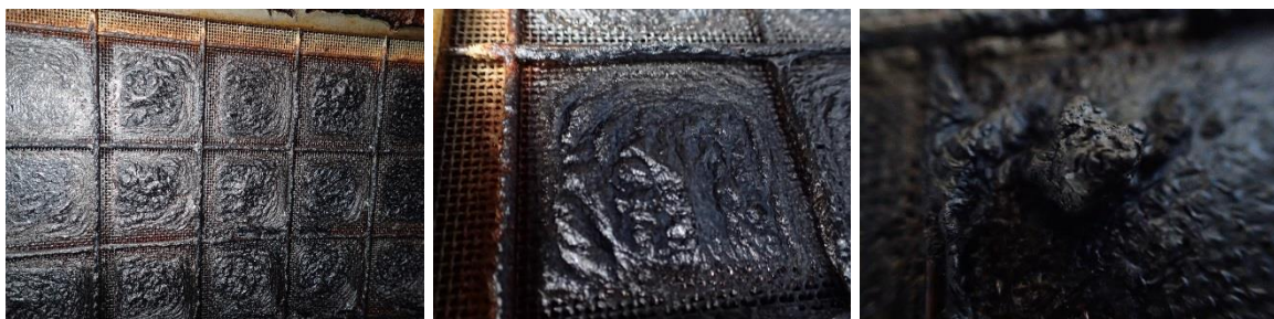
Figure 6 Inside of the 1130 \times 1130 \text{ mm} Flameless device after test BOX1-24 with 1000 \text{ g}/\text{m}^3 of cornstarch.
