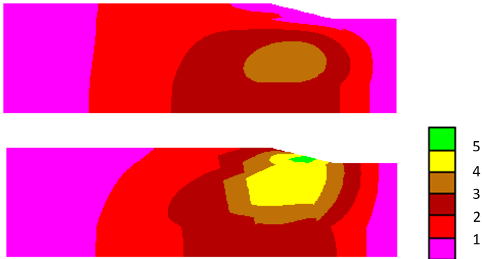
Figure 5: Horizontal displacements (cm) for the configurations (bottom) M1 with and (top) M0 without faults for stage 1
