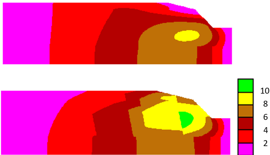
Figure 6: Horizontal displacements (cm) for the configurations (bottom) M1 with and (top) M0 without faults for stage 2
