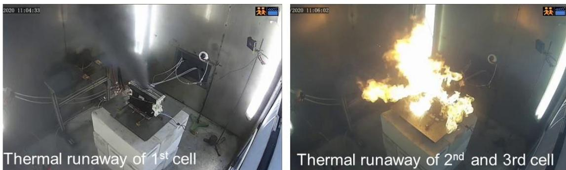
Figure 13: video extracts of the thermal runaway of the module
