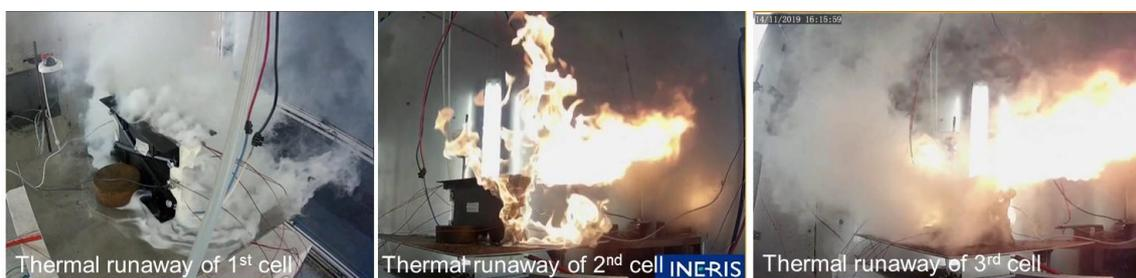
*Figure 9: video extracts of the thermal runaway of the 3 cells of the cluster*
