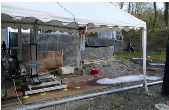
Fig. 11. Test 15 - Pictures showing the rain-out marks after the end of the release
