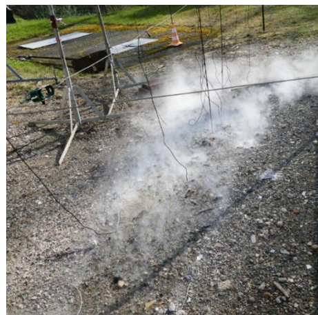
Fig. 11. Test 15 - Pictures showing the rain-out marks after the end of the release
