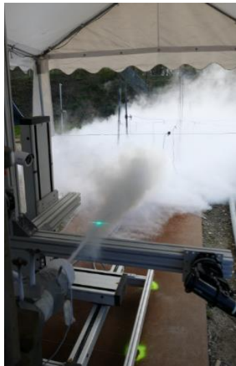
Fig. 10. Test 15 - Pictures revealing rain-out during the release
