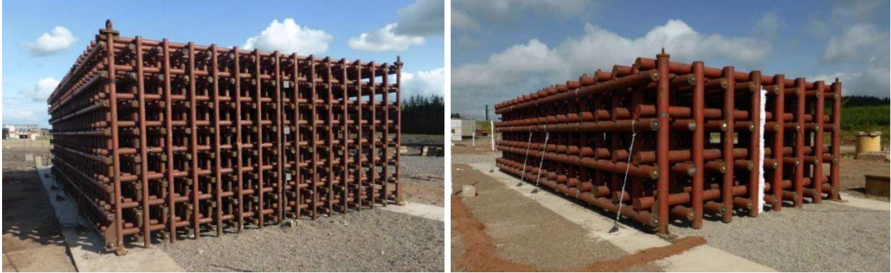
Fig. 2. The test rigs, with high (left) and medium (right) level of congestion, denoted as rig 7 and rig 8, respectively.
