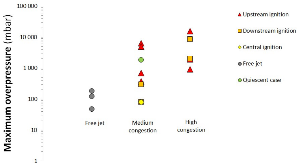
Fig. 3. Maximum explosion overpressures from all tests in the AIRRE campaign.
