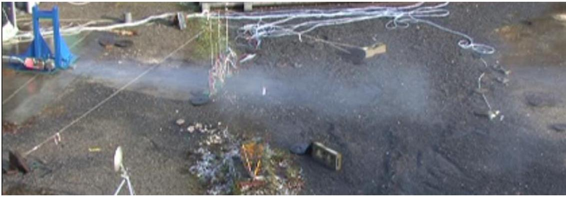
**Fig. 6.** View of an EXJET crawling jet (release diameter: 12mm, flowrate about 1 kg/s)
