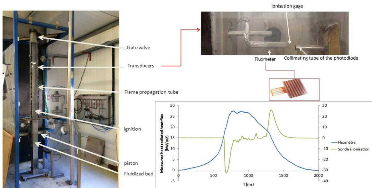
**Fig. 1.** Experimental setup and heat flux-ionisation gage signal for a stoichiometric  $CH_4$ -air flame
