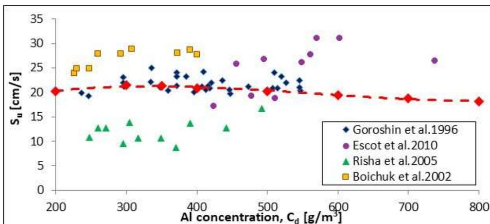
Fig. 6 : Laminar burning velocity in aluminium dust air mixtures (very small scale)
