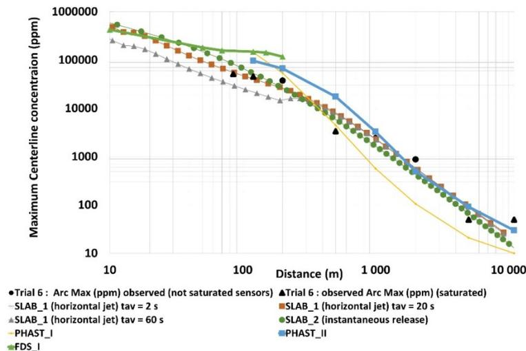
Figure 1.: Maximum arc-wise concentrations obtained for TRIAL 6
