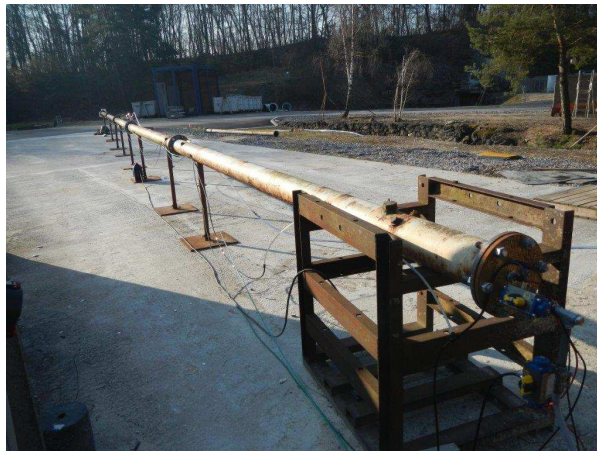
Figure 1: View of the experimental set-up. Top: PMMA pipe, with a 250-mm inner diameter. Bottom: metal pipe, with a 150-mm inner diameter.
