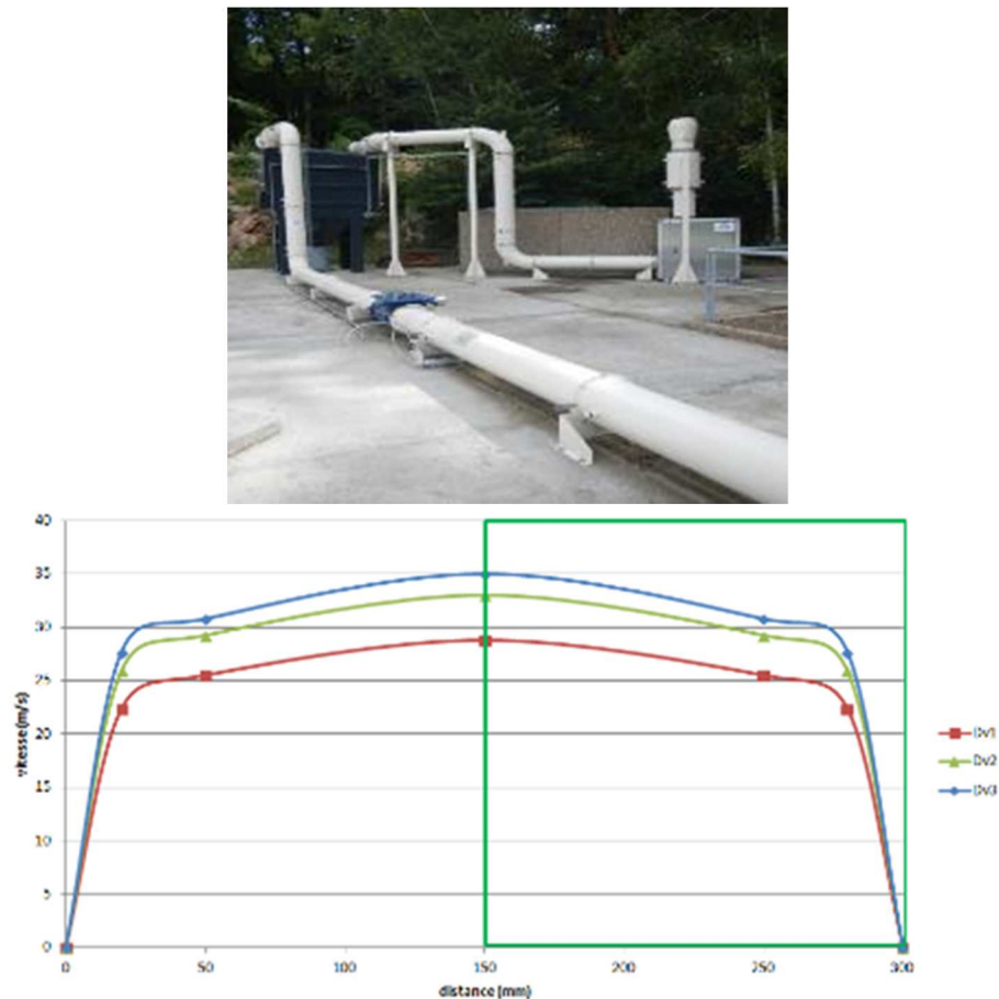
Figure 12 : Flow velocity measured in a 300 mm steel pipes (20 m long) in which the flow is established using a fan
