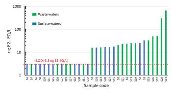
**Fig. 2.** *In vivo* measured 17β-estradiol equivalents (EEQ) expressed in ng/L for all the waste and surface water samples. The value of the limit of detection (LOD, red dashed line) of the EASZY assay was assigned for all inactive samples. (For interpretation of the references to color in this figure legend, the reader is referred to the web version of this article.)
