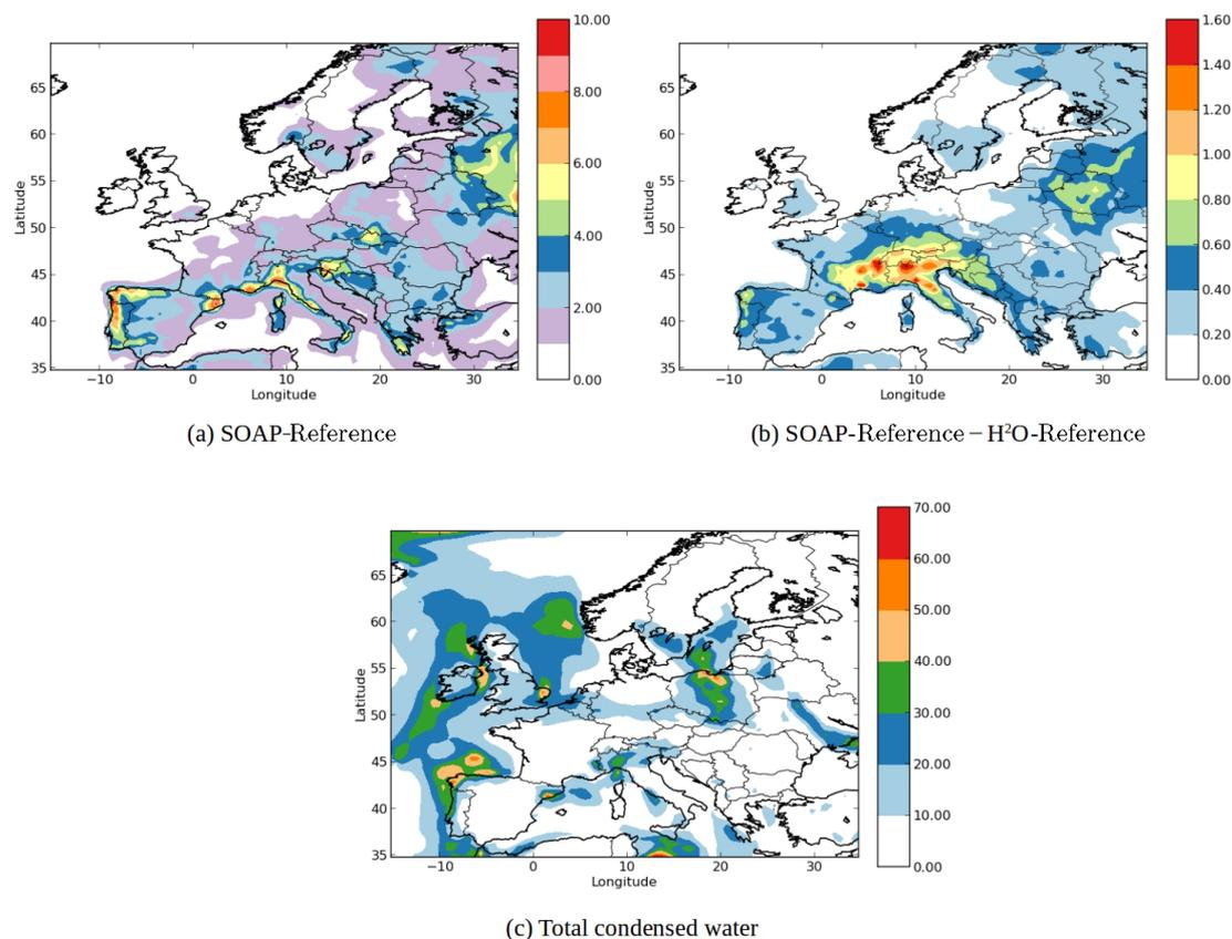
**Figure 4.** (a) SOA concentrations in the SOAP-Reference simulation ( $\mu\text{g m}^{-3}$ ), (b) the differences of the SOA concentrations between the SOAP-Reference and  $\text{H}^2\text{O}$ -Reference simulations ( $\mu\text{g m}^{-3}$ ) and (c) concentration of total condensed water in the SOAP-Reference simulation ( $\mu\text{g m}^{-3}$ ).
