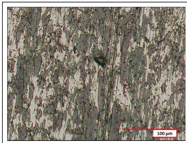
Figure 5. Disc track observed on optical microscopy when testing at 1.24 MPa of pressure and 25.0 m/s of speed (PV = 31 MPa.m/s).
