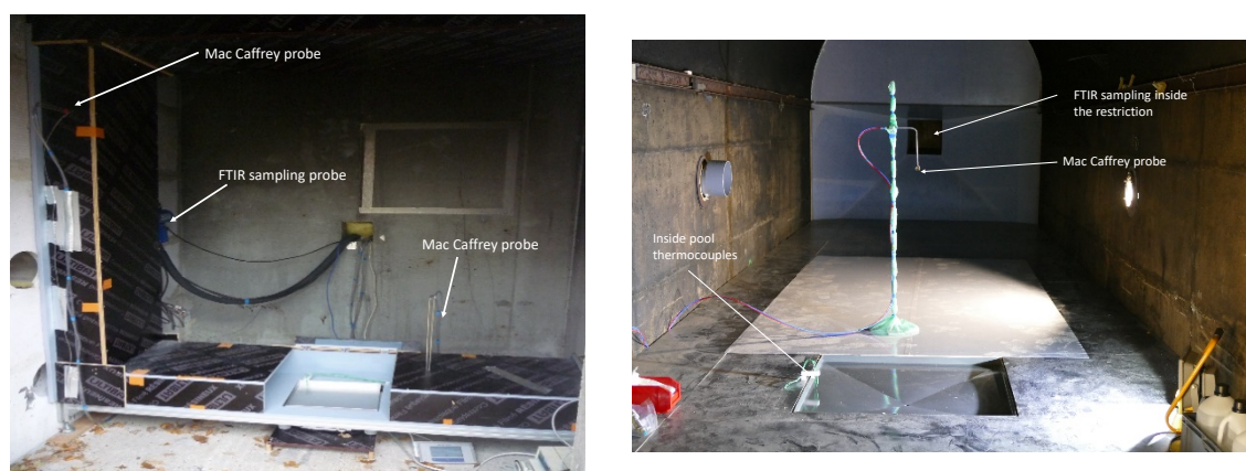
Figure 2. Picture of the pool photography and instrumentation for small ( left ) and medium ( right ) scales.
