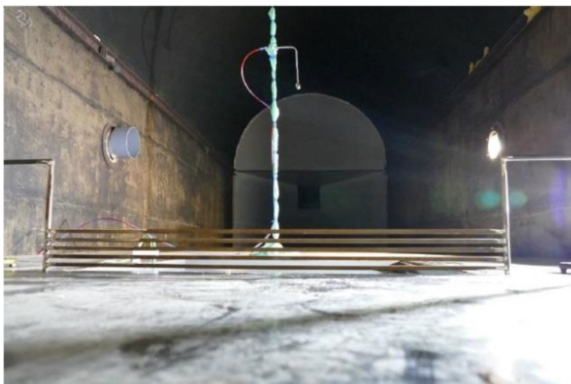
Figure 5. Picture of the system used to generate artificial turbulence upstream of the pool.
