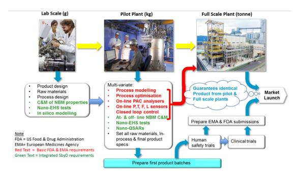
**Figure 3.** Integration of risk management framework into FDA/EMA 2003 Process Analytical Control Regulations for ATMPs (P = pressure, T = temperature, F = flow, L = level, PAC = process analytical control).
