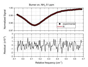
**Fig. 8.** Absorption signal and related fit, with the methane burner on, at an ammonia mixing ratio of 51 ppm (top), and residual, magnified by a factor of  $10^4$  (bottom)
