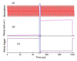
**Fig. 2.** Timing of the different signals: (a) Modulation at 1 MHz applied to the laser. (b) Current ramp at 1 kHz applied to the laser. (c) Trigger for the current ramp. All signals maintain the relative phases among themselves.
