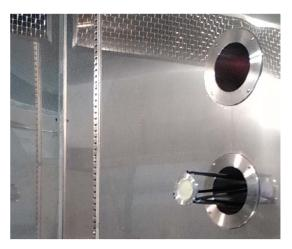
**Fig. 7.** Photo of the multipass cell inside the climatic chamber for the test of temperature stability.
