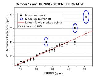
Fig. 11. Correlation of second derivative measurements with INERIS FTIR analyser.
