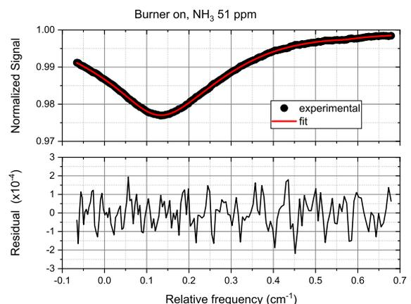
**Fig. 8.** Absorption signal and related fit, with the methane burner on, at an ammonia mixing ratio of 51 ppm (top), and residual, magnified by a factor of 10<sup>4</sup> (bottom).
