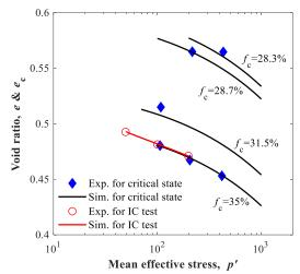
Figure 4 Isotropic compression curve and critical state line in the  $e - \log p$  plane
