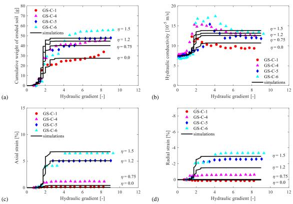
Figure 9 Comparisons between predicted and experimental results of erosion tests (a) Cumulative eroded soil mass; (b) hydraulic conductivity; (c) axial strain and (d) radial strain
