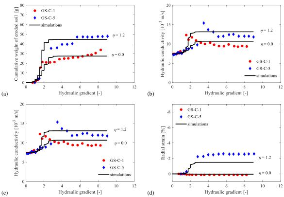
Figure 7 Comparisons between simulated and objective experimental results of erosion tests (a) Cumulative eroded soil mass; (b) hydraulic conductivity; (c) axial strain and (d) radial strain
