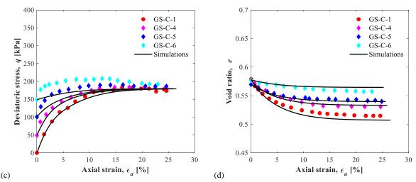
Figure 10 Comparisons between predicted and experimental results of triaxial tests (a,c) deviatoric stress versus axial strain and (b,d) void ratio versus axial strain. Hollow points indicate triaxial compression of the initial specimen, and solid points indicate triaxial compression of eroded samples.
