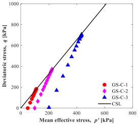
Figure 5 Stress path of drained triaxial tests
