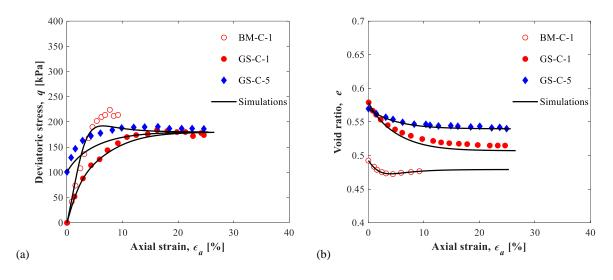
Figure 8 Comparisons between simulated and objective experimental results of triaxial tests (a) deviatoric stress versus axial strain and (b) void ratio versus axial strain. Hollow points
