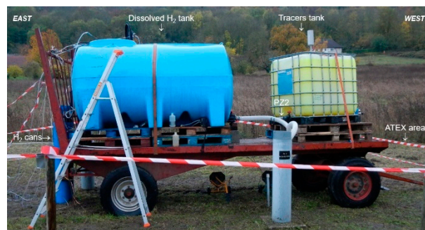
Figure 5. View of the injection device.
