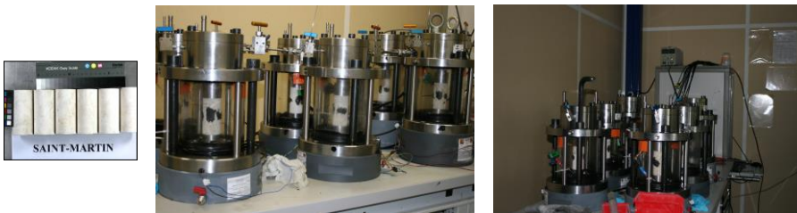
Figure 2. Experimental device used for creep tests with controlled relative humidity.
