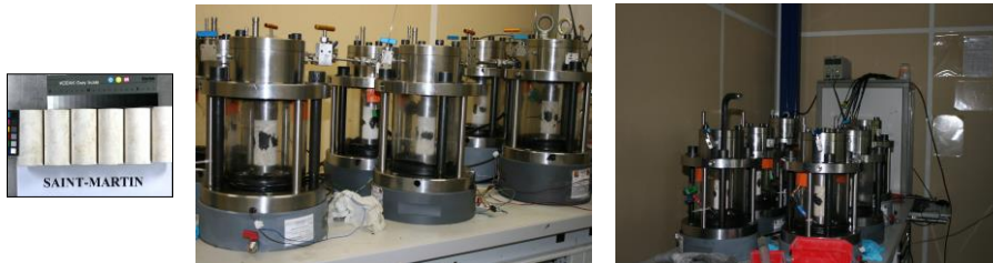
Figure 2. Experimental device used for creep tests with controlled relative humidity.
