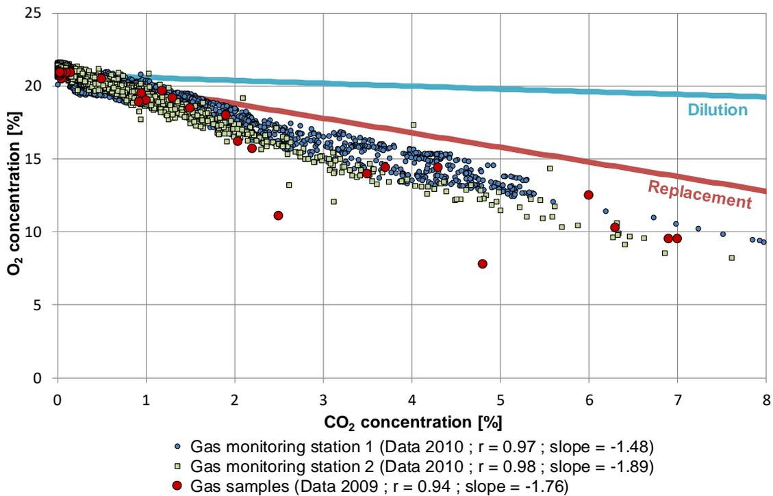
Figure 2. O<sub>2</sub> versus CO<sub>2</sub> concentrations measured in situ by sampling or continuous monitoring.
