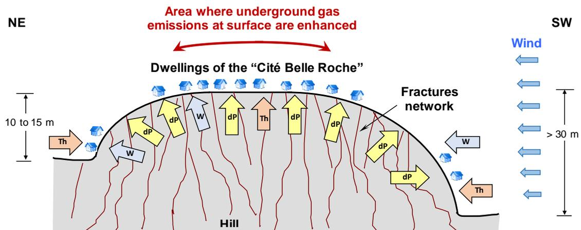
Figure 5. Schematic diagram of the combined action of a depression (dP; yellow arrows), thermal draught (Th; orange arrows) and prevailing wind (W; blue arrows) in the “Cité Belle Roche” during winter.
