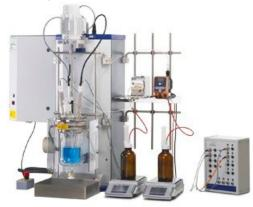
Picture 1. Picture of reaction calorimeter RC1.
