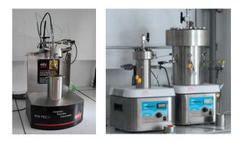
Picture 2. Pictures of Phi-Tech I (a), ARSST (left) and VSP II (right) (b).
