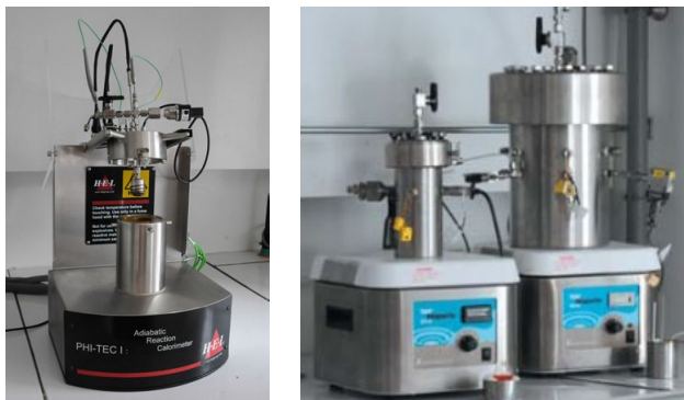
Picture 2. Pictures of Phi-Tech I (a), ARSST (left) and VSP II (right) (b).
