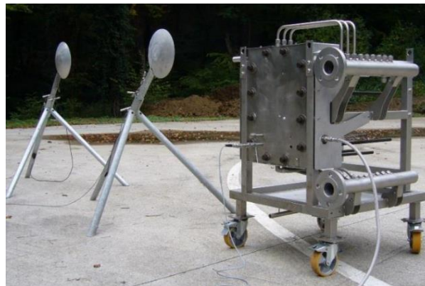
Picture 2: Test installation with atmospheric pressure sensors and pressure sensor on the SiC plate (middle of the picture). The cameras are not visible on the picture.
