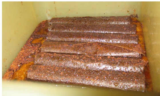
Picture of degraded dynamite cartridges with presence of exudate
