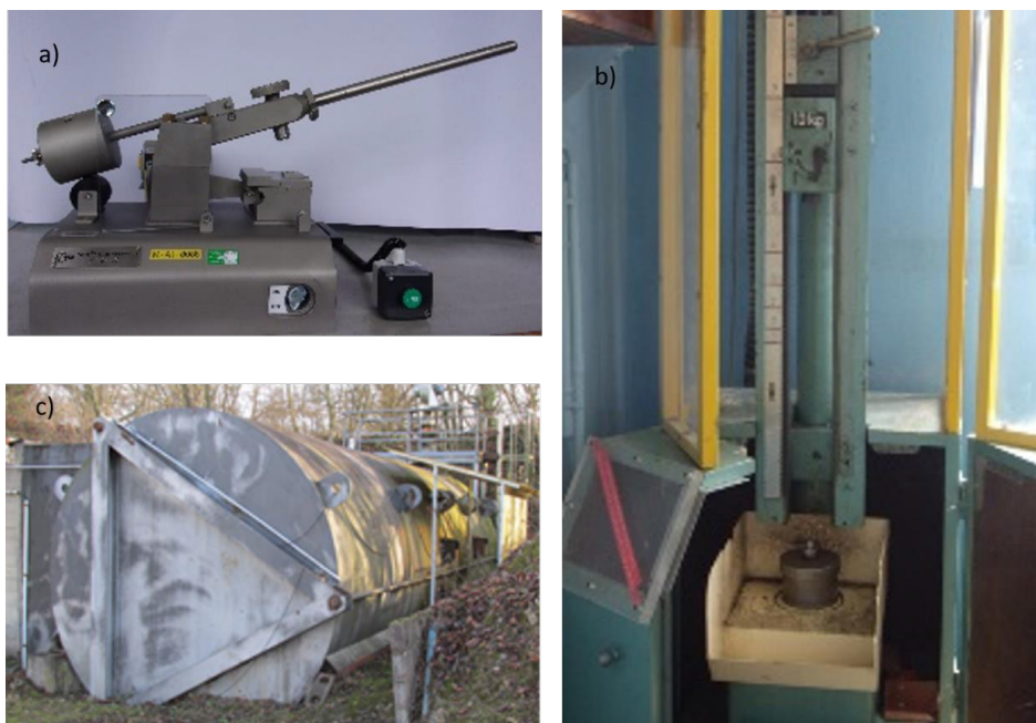
Figure 3: Some apparatus to test explosive properties a) sensitiveness to friction; b) sensitiveness to impact c) blast chamber of 50 m 3
