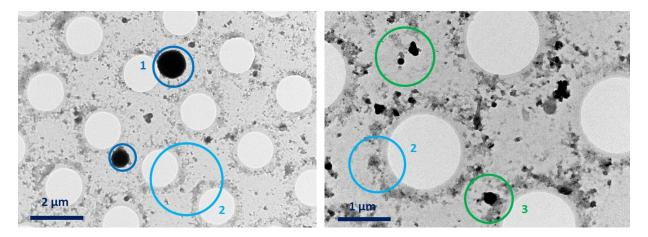
Figure 7. TEM analysis of the aerosol generated when incinerating the PVC waste. Three categories of particles were identified.
