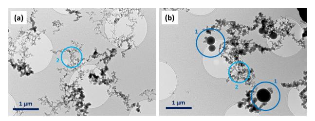
Figure 4. TEM analysis of the aerosol generated when incinerating the PDMS waste with two different temperatures: 850 °C (a) and 1100 °C (b). Two categories of particles were identified.
