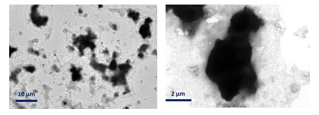
Figure 8. TEM analysis of the combustion residue of the PVC. The residue was mixed with water and alcohol and a droplet was deposited on TEM grid prior to analysis.
