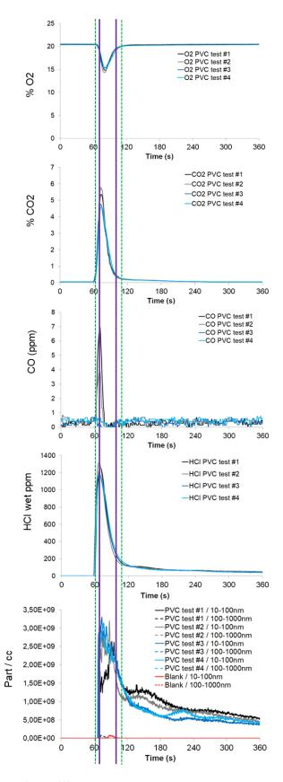
Figure 6. Temporal evolution of the different gases  $(O_2, CO_2, CO \text{ and } HCl)$  and of particle emission when incinerating the PVC waste.
