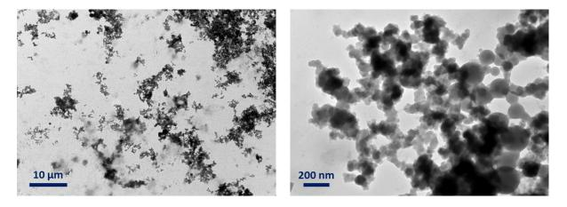
Figure 5. TEM analysis of the combustion residue of PDMS. The residue was mixed with water and alcohol and a droplet was deposited on TEM grid prior to analysis.
