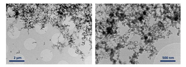
Figure 12. TEM analysis of the aerosol generated when incinerating the mixture of the three wastes.
