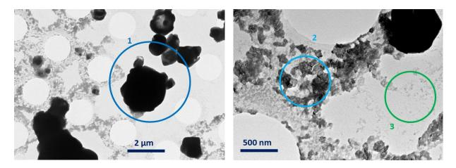
Figure 10. TEM analysis of the aerosol generated when incinerating the resin waste. Three categories of particles were identified.
