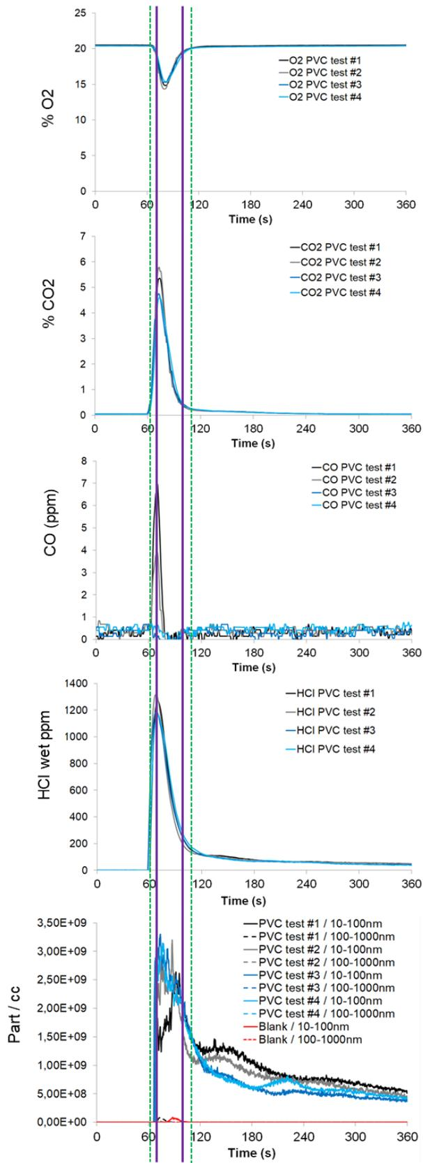
Figure 6. Temporal evolution of the different gases (O<sub>2</sub>, CO<sub>2</sub>, CO and HCl) and of particle emission when incinerating the PVC waste.
