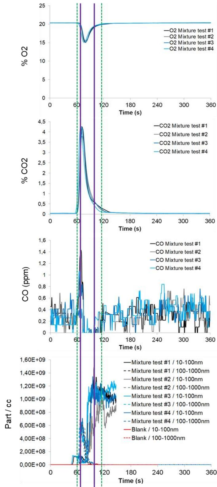
Figure 11. Temporal evolution of the different gases (O<sub>2</sub>, CO<sub>2</sub>, CO) and of particle emission when incinerating the mixture.
