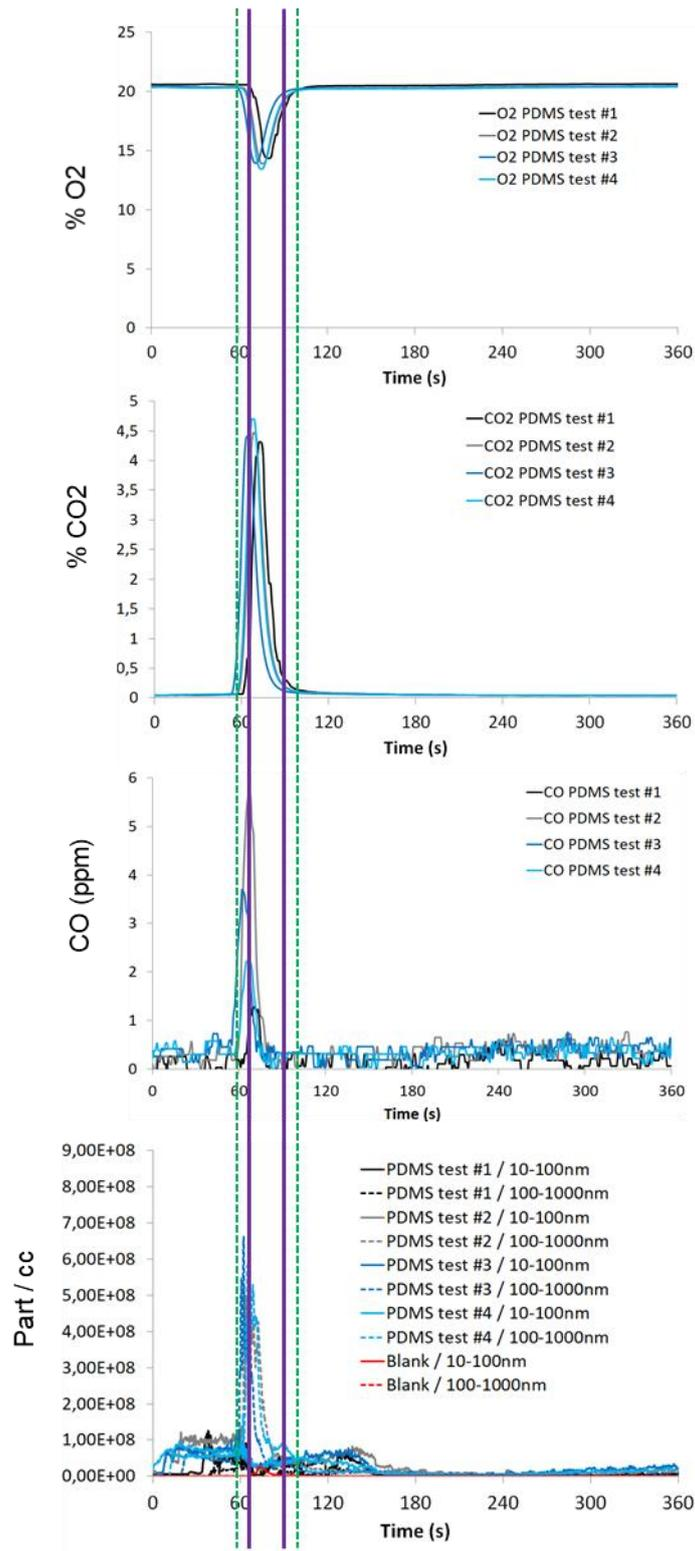
Figure 2. Temporal evolution of the different gases (O<sub>2</sub>, CO<sub>2</sub>, CO) and of particle emission when incinerating the PDMS waste.
