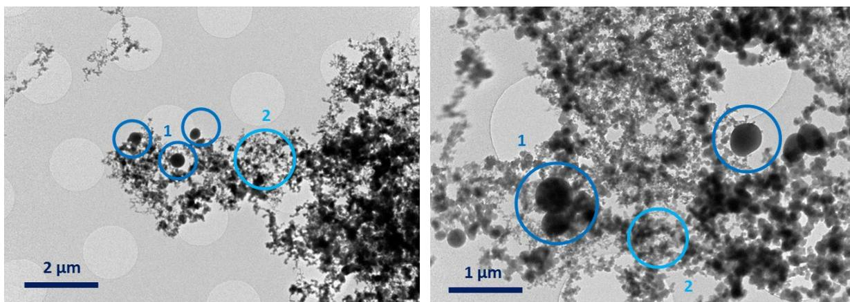
Figure 3. TEM analysis of the aerosol generated when incinerating the PDMS waste. Two categories of particles were identified.
