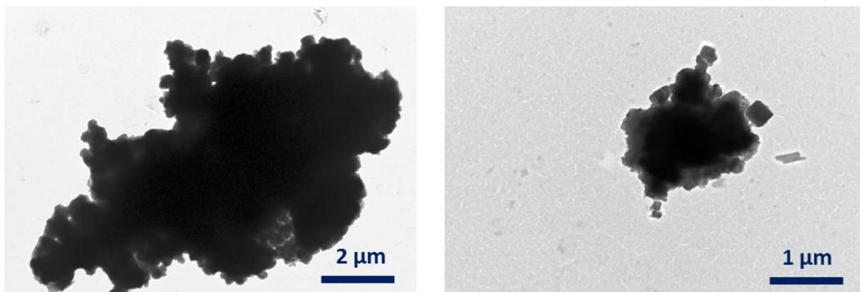
Figure 13. TEM analysis of the combustion residue of the mixture of the three wastes. The residue was mixed with water and alcohol and a droplet was deposited on TEM grid prior to analysis.
