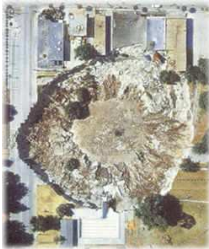
Figure 1. Land subsidence (sinkhole) in Central Kansas related to underground rock dissolution (after USGS water science).
