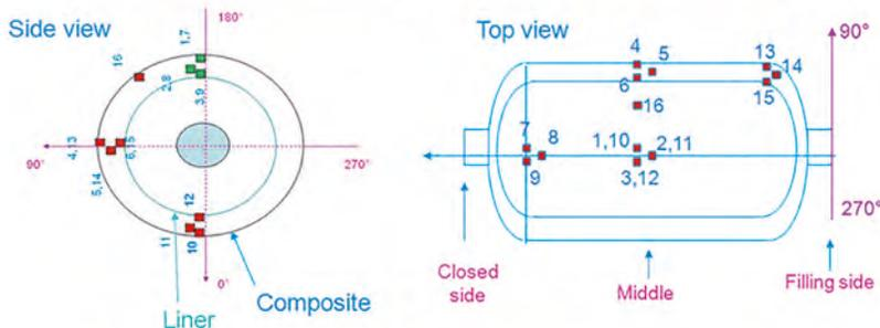
■ 2,8 → Means that thermocouples 2 and 8 are superposed in this view
