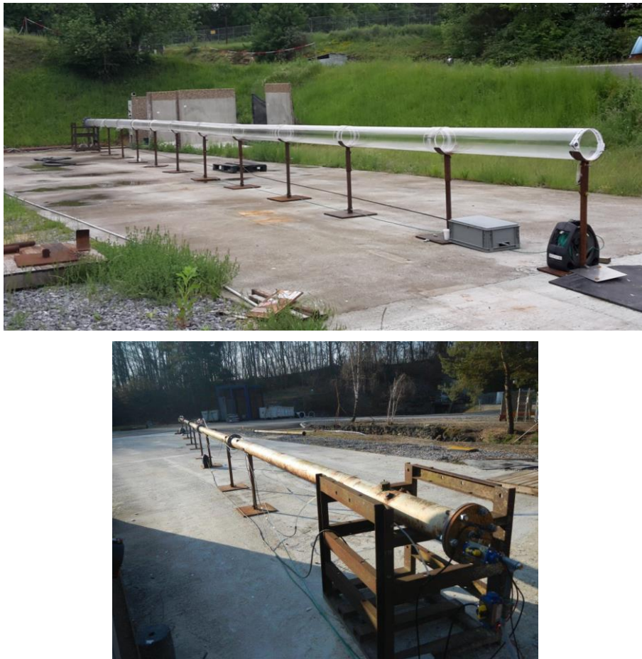
Figure 1: View of the experimental set-up. Top: PMMA pipe, with a 250-mm inner diameter. Bottom: metal pipe, with a 150-mm inner diameter.
