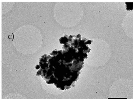
Figure 9 c): Micronic NOAA and nano-TiO<sub>2</sub>, or nano-pigment. Scale 1  $\mu$ m.
