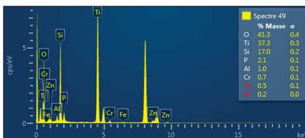
Figure 10 : EDS analysis of the Figure 9 c)
