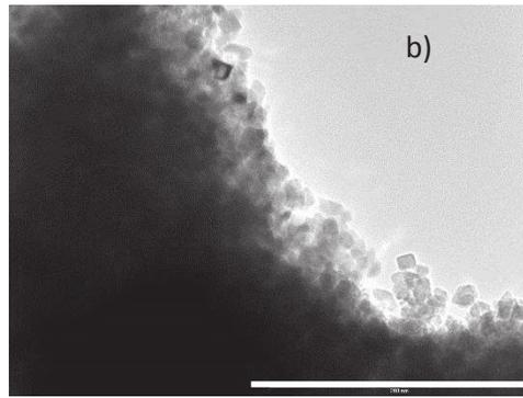
Figure 8 a) nano-TiO<sub>2</sub> particles (7-30 nm) nano-pigment and particles of SiO<sub>2</sub> presents on the sample. Scale 100 nm. b) under agglomerate form, nano-TiO<sub>2</sub> shape is also irregular compared to nano-pigment. Scale 200 nm.
