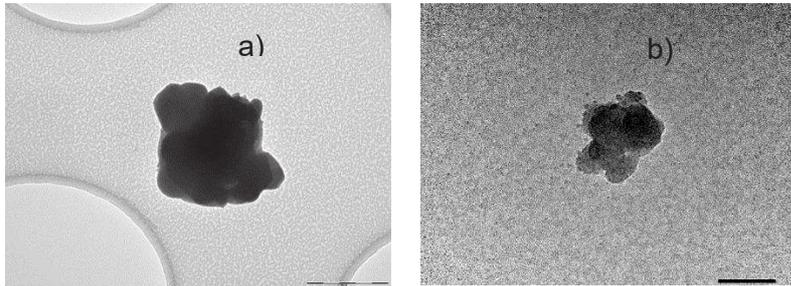
Figure 1 a) submicronic particles from P2, scale 200 nm. b) Nano-TiO<sub>2</sub> particles around a NOAA are detected on P2 samples. They are made of isolated primary particles of 7 nm, scale 100 nm.
