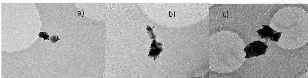
Figure 11 : NOAA of TiO<sub>2</sub> (~ 100 nm size) and debris of paint matrix are detected among collected objects. a) scale 500 nm, b) scale 300 nm and c) scale 500 nm.
