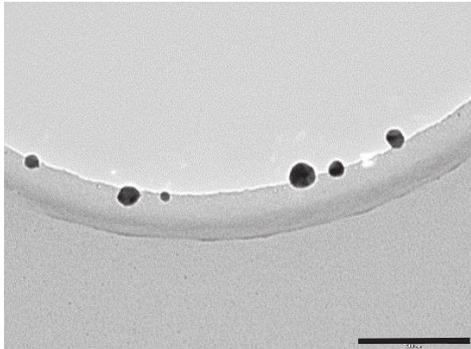
Figure 7 : nano-pigments of TiO<sub>2</sub> presents on the sample. Scale 200 nm.
